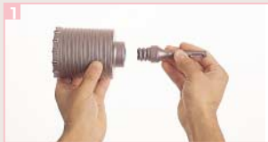
1 Screw the shank into the core drill body.
